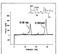
Figure 3. Stretching and relaxation force curves indicating the irreversible process of helix unfolding.
