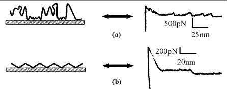
Figure 1. From adsorption conformation to force curve profile. (a) Typical force profile of PVP on amino modified substrate. (b) Typical force profile of PDDA on sulfonic modified substrate.
