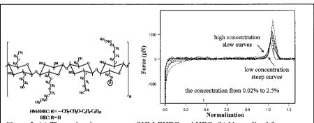
Figure 2. (a) The molecular structure of HM-EHEC and HEC. (b) Normalized force curves of HM-EHEC obtained under different concentration.
